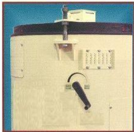
Handle for adjustment of stones
