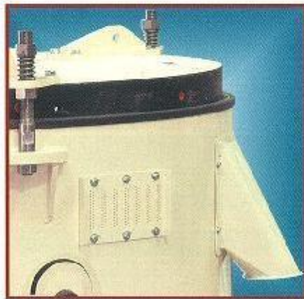
Air intake and flour outlet
